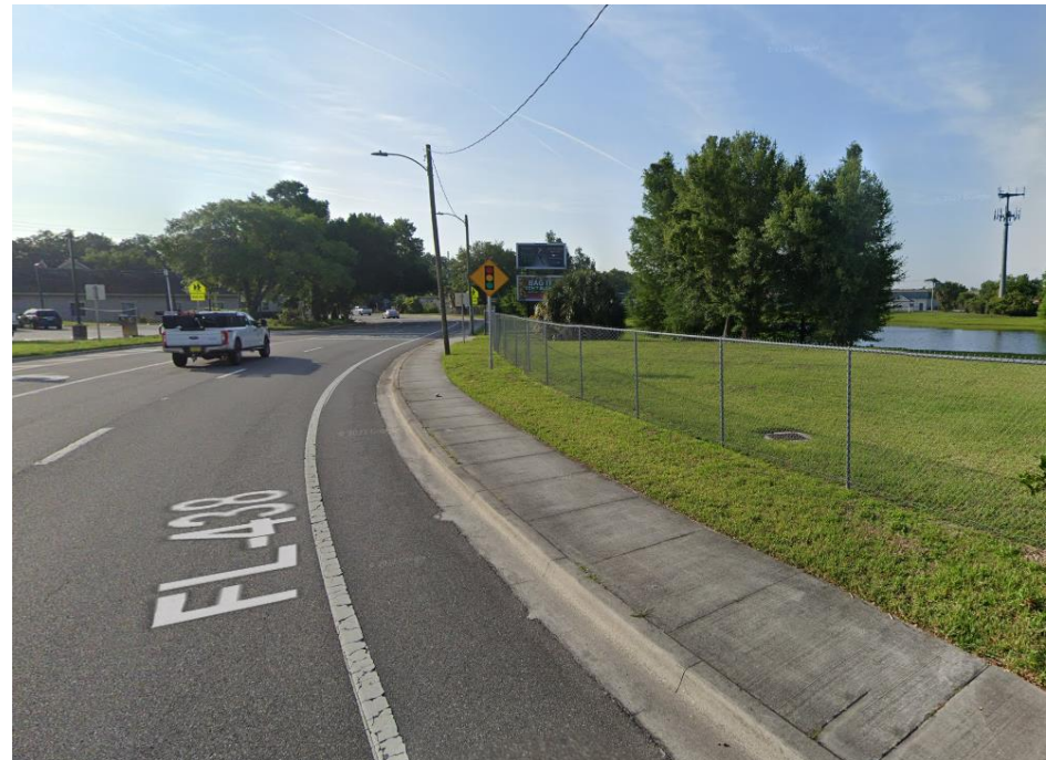
Countermeasure #6: This project would combine the bike lane and sidewalk, resulting in a multi-use path on the south side of Princeton Street. The fence to the south could be removed in order to plant trees on the City of Orlando-owned parcel shown above. This strategy would improve bike-ped comfort and safety.
